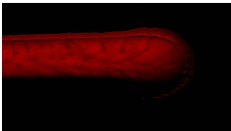
**Figure 3.** Fluorescence imaging of microchannel with GdVO<sub>4</sub>:Eu<sup>3+</sup> under excitation of 265 nm
