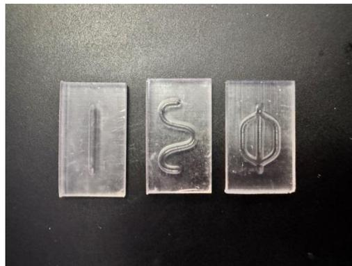
**Figure 2** Printed microfluidic devices
